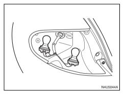
To replace a tail/stop lamp or a rear turn signal lamp bulb:
